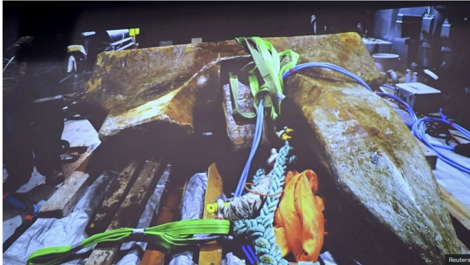
A Finnish Border Guard's photo of an anchor that may have damaged the pipeline
